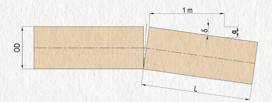
$\delta$  Maximum angular deflection in degrees (°) α Maximum angular deflection im millimeters per metre (mm/m)
