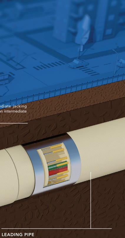
For intermediate jacking station arrangements, the movable structure of the leading pipe is utilized. The structure of the leading pipe is designed with a groove on one end so that it moves in accordance with the extension and retraction movements that may occur in the intermediate jacking station during assembly.
